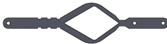
Figure 18 Example of one of the linear bistable elements. Adapted from [75].
