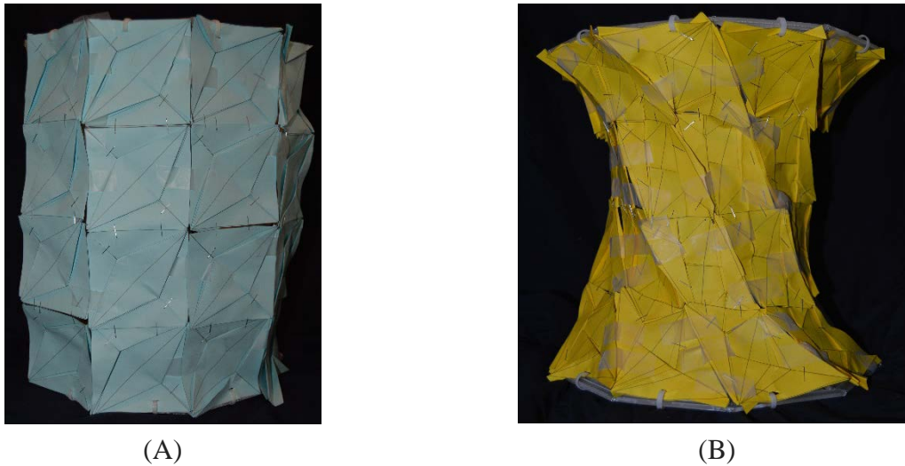
Figure 32 Undeformed (A) and deformed (B) mechanism, with unit strips of the origami mounted to it
