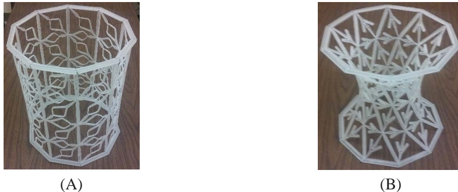
Figure 17 The mechanism in the undeformed state (A), which forms a cylinder, and the deformed state (B), which forms a hyperboloid. Adapted from [75].
