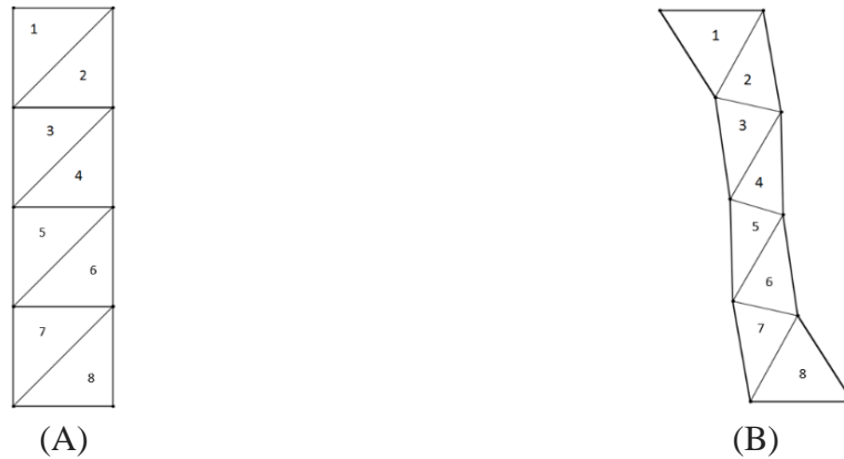
Figure 20 Simplified model of the unit strips. (A) is undeformed and (B) is deformed.
